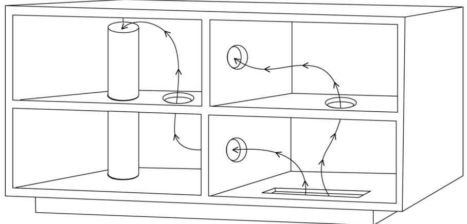
this will result in less back-to-front air movement. If one side of the cabinet is visible, and the owners don't want it used for ventilation, it's time for a frank discussion of the consequences of not providing ventilation. The thought of replacing equipment every few months may have a chilling (pun intended) effect....!
