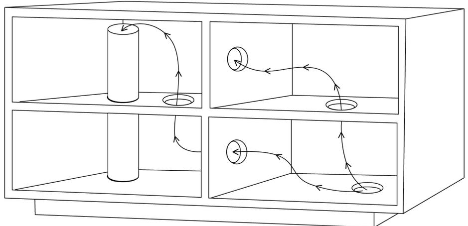
the floor itself so that you can create a “snorkel” running from just an inch or so below the top of the cabinet down into the lower level where it can be attached to the intake (suction) side of an Active Thermal Management Cool-cube®, ordered with 4” flex tubing.
